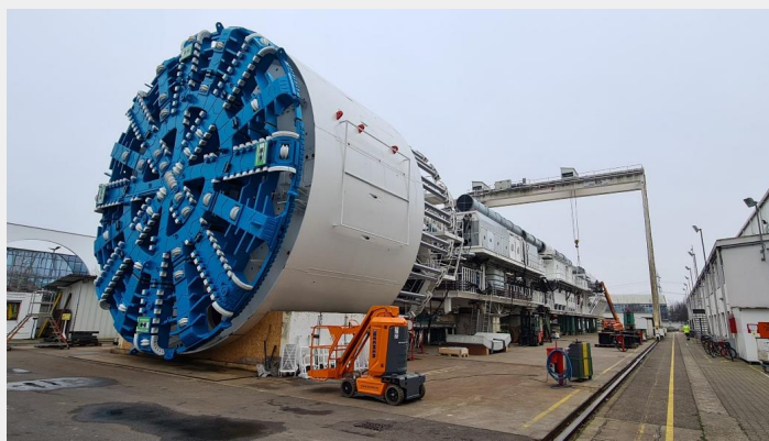
Fig.1: Silvertown Tunnel TBM following factory acceptance test Fig.2: First parts (TBM tailskin) being delivered to site
