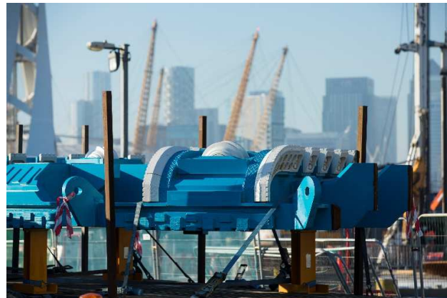
Fig. 2 The cutterhead of the TBM
