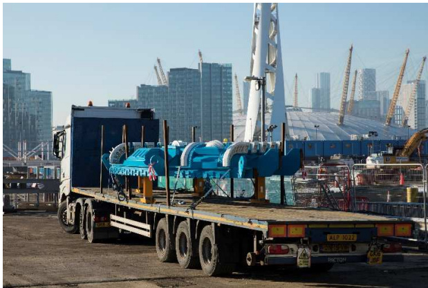
Fig. 1 transportation of TBM parts
